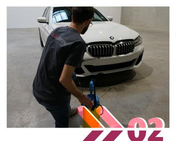
Spray soapy water / gel on the part of the body to be protected. This operation makes it easier to place the vinyl on the vehicle. Check that there are no dust remaining before wetting the bodywork, otherwise clean the surface again before starting the installation
