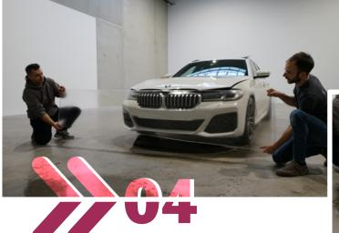
Place the Protector Ultra Top on the bodywork and stretch it to ensure it perfectly takes the surface's shape that needs to be covered
