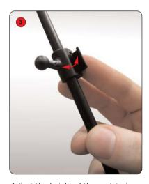
Adjust the height of the eyelet pip on each leg by opening up the lever on the fixing, moving to desired position and then closing the lever to secure.
